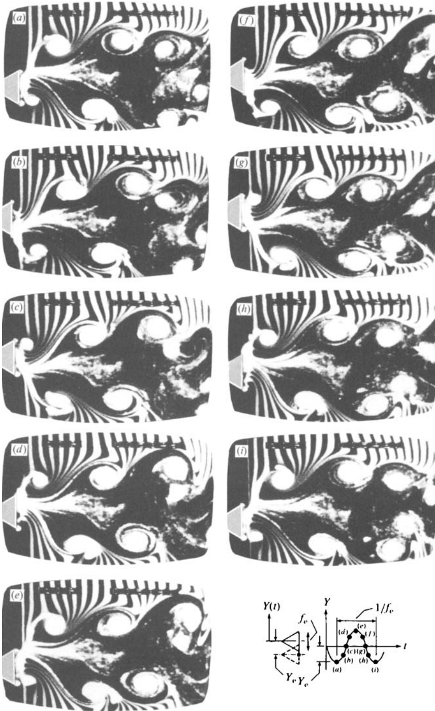
FIGURE 9. Mechanisms of small-scale vortex-vortex interaction for case of superharmonic excitation at f_e/f_0^* = 2 . Y_c/D = 0.30 .
