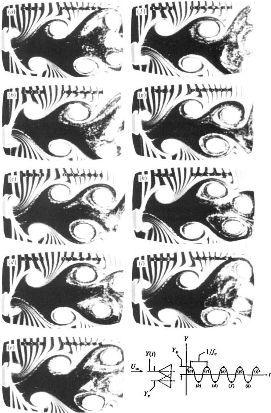
FIGURE 8. Mechanisms of small-scale vortex-vortex interaction for case of non-harmonic excitation at f_e/f_0^* = 1.5 . Re_D = 855 ; Y_e/D = 0.30 .
