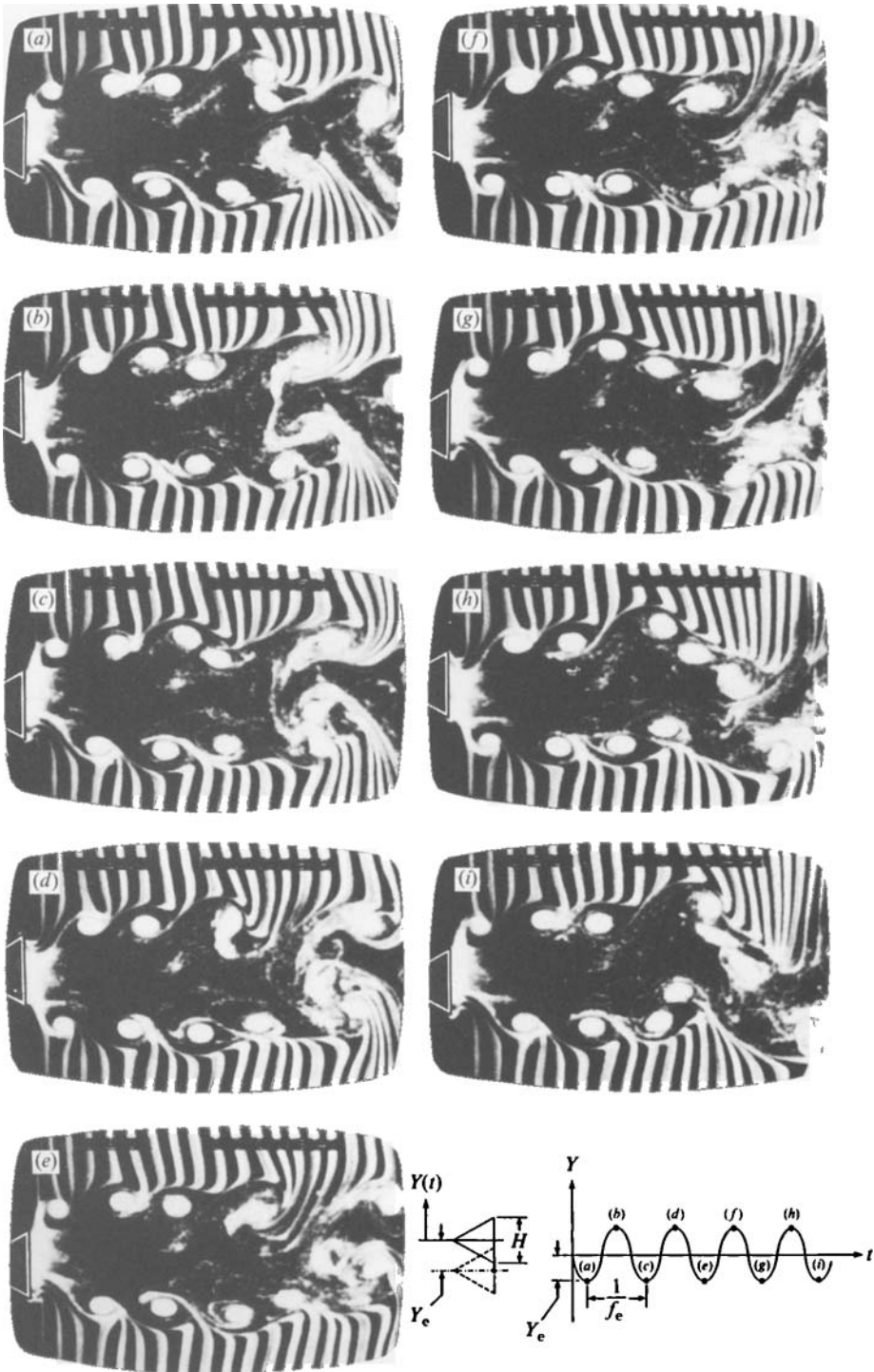
FIGURE 10. Mechanisms of small-scale vortex-vortex interaction for case of superharmonic excitation at f_e/f_0^* = 4 . Re_D = 855 ; Y_e/D = 0.13 .
